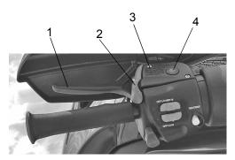
**Tip:** If the brake lever is squeezed tightly enough, the lock will move freely into place. Do not force the lock or it may break.
